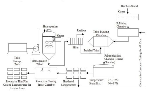
Figure 10: Process Flow Diagram for the Production of Protective Thin Film Coated Lacquerwares
